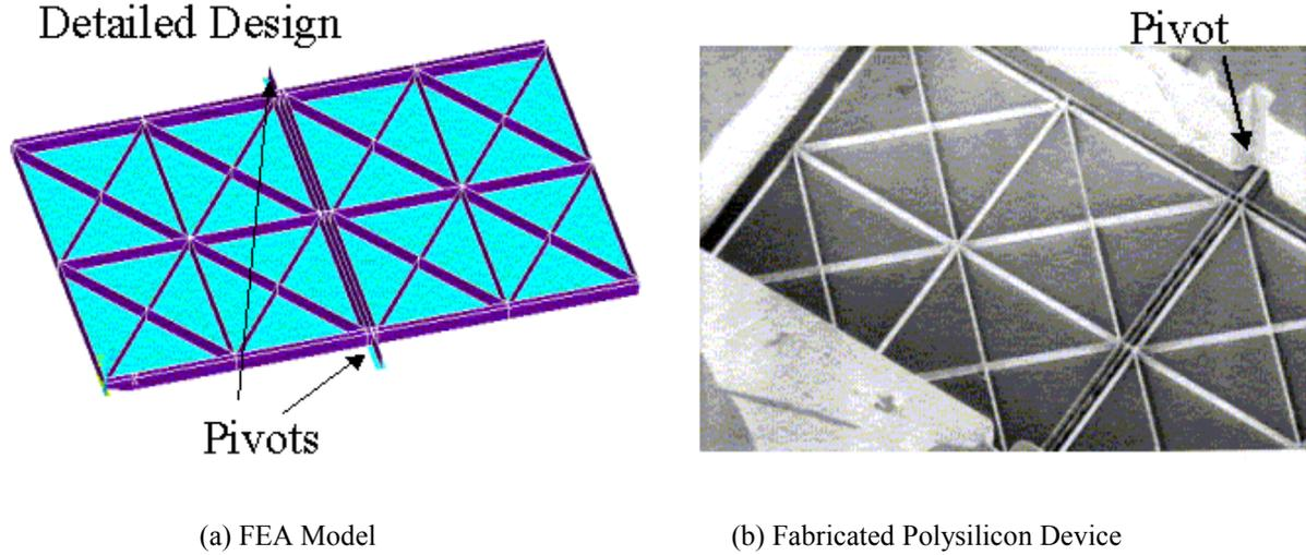
Figure 3. Diaphragm Structure of the Ormia Differential Microphone
