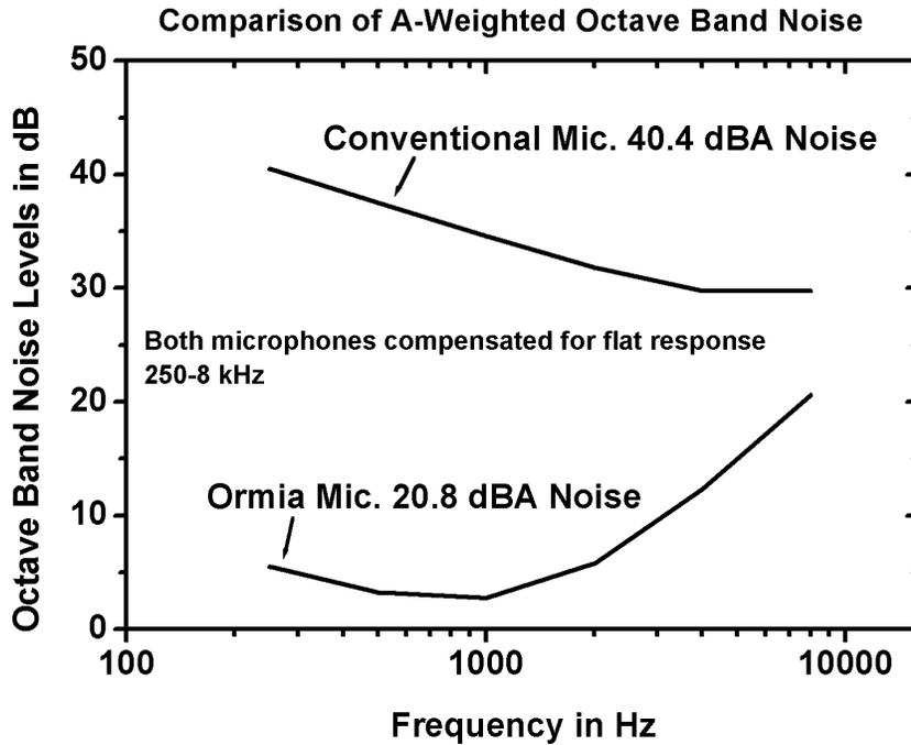
Figure 5. Predicted Output Noise Spectra of the Differential Microphones
