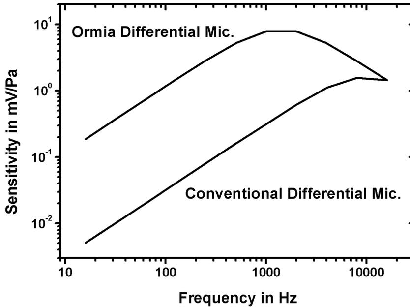
Figure 4. Predicted Frequency Responses of the Differential Microphones
