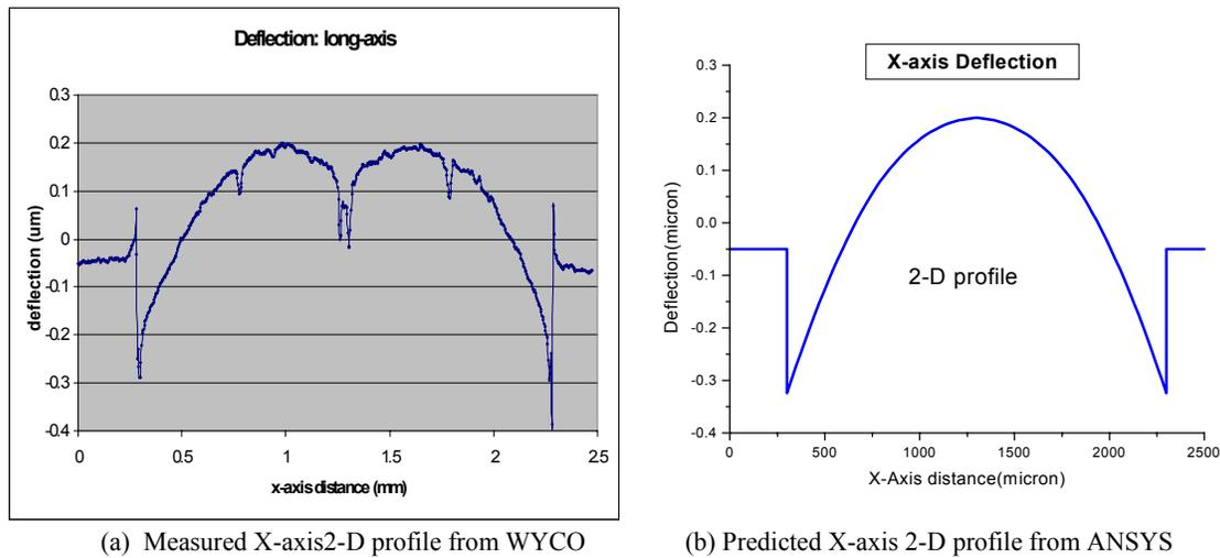
Figure 6. Static Deformation Along the 2 mm Long Axis
