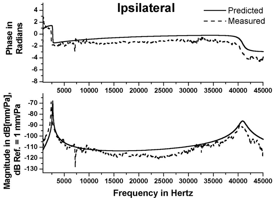
Figure 8. Comparison of measured and predicted response of our differential microphone diaphragm (with no backplate) due to an incident sound. Data are normalized relative to the incident sound pressure.
